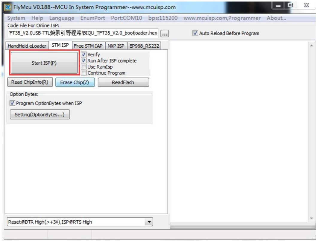
9. The bootloader flashing is finished
