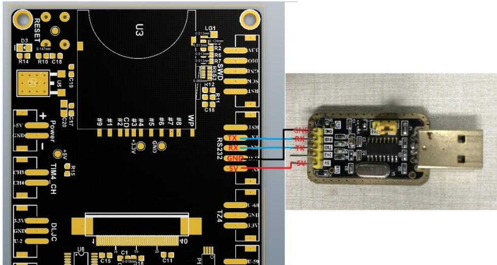
3. Install the CH340 driver software (You can find it in internet), then connect the TFT35 and CH340 debugger module to the computer.
